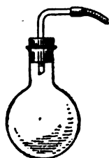
Fig. 1.—Apparatus for showing the weight of air.
